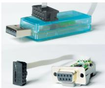
The abbreviation UART stands for Uni-ver-sal Asynchronous Re-ce-i-ver/Tran-smit-ter. It is a serial data interface with a defined speed. Regardless of the actual voltage level of the RS232 signals, these RS232/RS482 devices present signals to the microcontroller as a logical 0 or 1.
