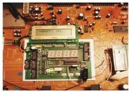
Integrated circuits within telecommunications and industrial electronic devices and complex consumer devices (for example, in a TV set) often communicate using the I2C protocol. This article describes a simple device that can monitor traffic on the I2C bus. Let's find out what kind of messages these chips exchange!
