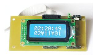
Some AVR microcontrollers have Timer2 which can operate in asynchronous mode. These AVRs are the ATmega8, ATmega168 and ATmega16 etc. With some help from simple Bascom code, one can make an accurate clock which will display date and time.
