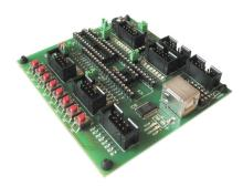
MiniPin II is a smaller brother of MegaPin. Smaller, but still very user friendly and versatile development board, where programs for AVRs may be tested and evaluated. Connecting your programmer to the MiniPin II board.
