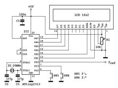
The ATtiny2313-based frequency reference produces a series of rectangular pulses with a 50% duty cycle. The frequency of these pulses is very stable, while the frequency range covers a full 10 decades, ranging from 0.001 Hz to 10 MHz.
