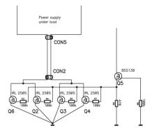
Neither of the choices mentioned above is too cost-effective for an electronic hobbyist, so we need a different approach. While testing the PWM power supply, I tested my first prototype of a PWM electronic load, consisting of a MegaPin board and one MOSFET power transistor. That prototype proved the concept very well. Using a selection of different output transistors I could select a resistance in the range of a couple of Ohms down to milliOhms.
